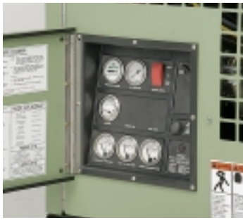
Curbside Instrument Panel Hinged, padlockable door.
