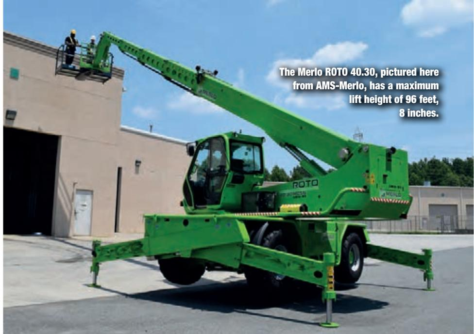
The Merlo ROTO 40.30, pictured here from AMS-Merlo, has a maximum lift height of 96 feet, 8 inches.
