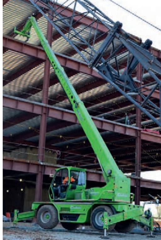
**The Merlo ROTO 45.21 MCSS, pictured here, has a lifting capacity of 10,000 pounds.**
