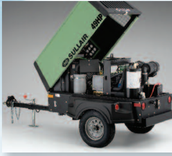
Clam Shell Canopy Compact/Lightweight design.
